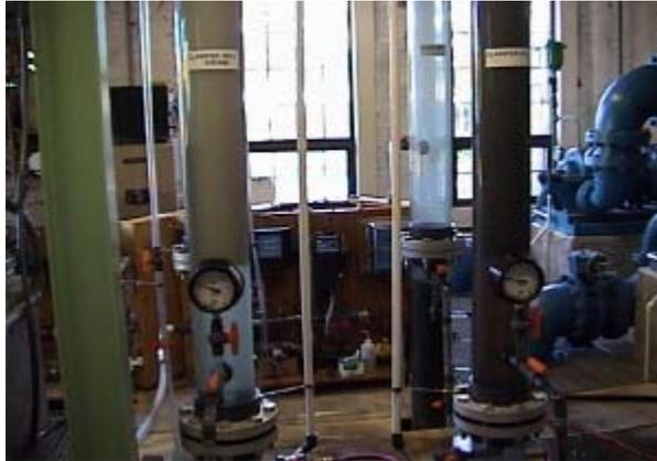
Parallel process comparison for adsorber clarifiers followed by Mixed Media Filters on right compared to Ozone plus coagulants (on left).
